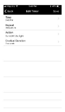
5. The controller has a build in timer function. To do so, press on the top right, next to ON/OFF, switch the clock icon. Then the selection menu will be shown with time, Repeat (Mon-Sun),
