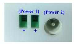
Power 1: Adopt wire plug-in and screwing terminal power input
