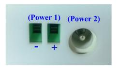
Power 1: Adopt wire plug-in and screwing terminal power input Power 2:Adopt the DC female Connector.
